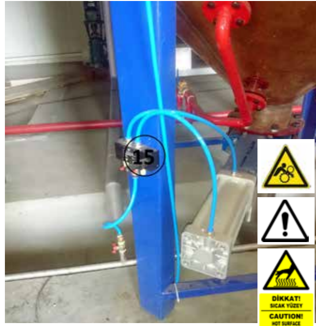
15. When the distillation process is completed, it is used for disposal of the pulp in the unit. Use after checking that door 2 is opened.
